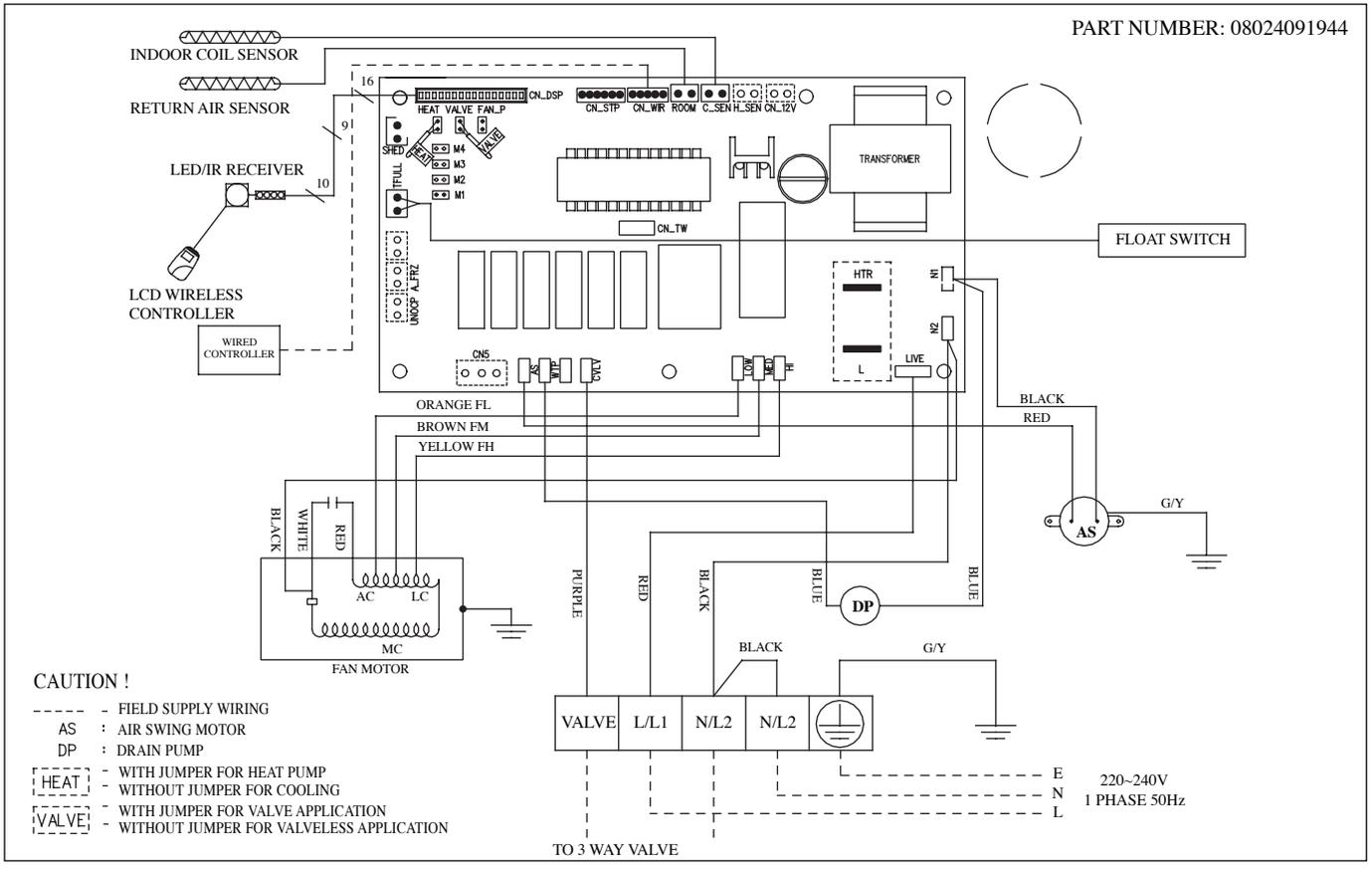
**Note :** Unit comes in standard heatpump and for valve application.
