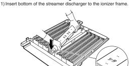
2) Insert top of the streamer discharger.
