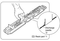
\*1 Wipe off only the resin part. \*2 Do not touch the discharge needle. Bending the needle will reduce deodorizing performance
