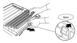
2. Attach the streamer discharger.
