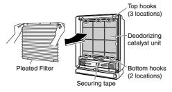
2) Take out a new pleated filter (1 sheet) and then attach it to the deodorization catalytic unit.
