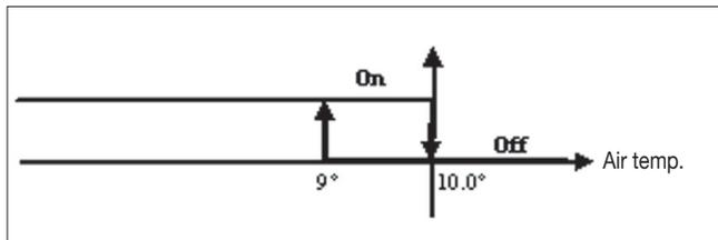
When temperature exceeds 10°C the thermostat will resume the Off status.
