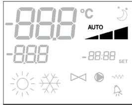
**NB:** if the active speed is different from the one selected by the user (in the case of a forced override), pressing the button
