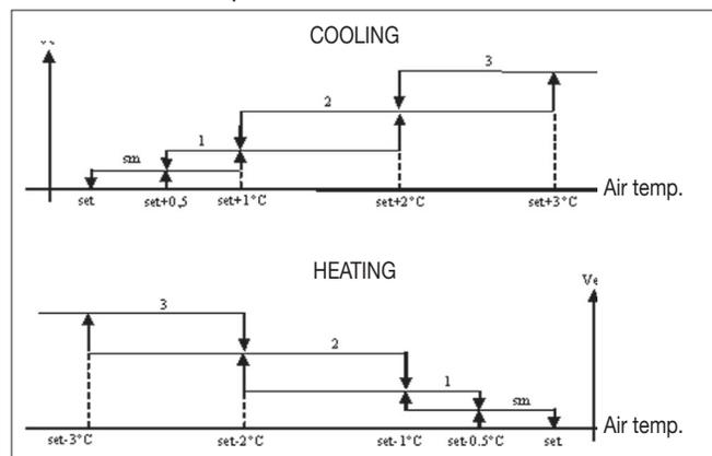
**NB:** in case of 4-speed configuration and valve, or 3-speed configuration + CN (natural convection), ventilation in heating mode is shifted by 0.5°C to permit a natural convection phase
