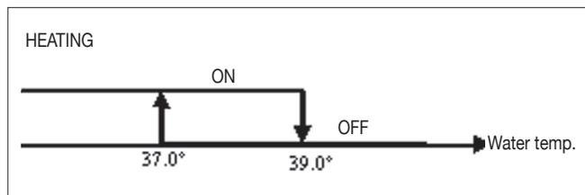
Enabling of the heating element is tied to the water temperature. The related enabling logic is described below. The enabling signal will not be given if the water sensor is either not present or disconnected
