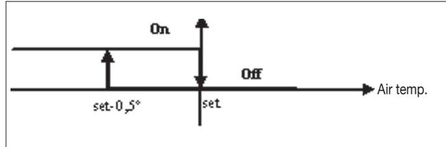
If use of the heating element is selected by the user, it will be activated on a call from the thermostat based on the room temperature
