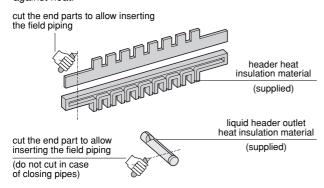
Apply the heat insulation material and seal all connections with tape.
