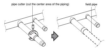
Use the supplied reducer/expander pipes when necessary
