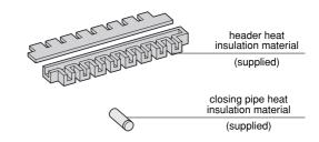
Apply the heat insulation material and seal all connections with tape.
