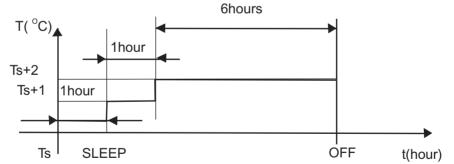
b.After setting the sleeping function, the heating mode will run as per the following rules:
