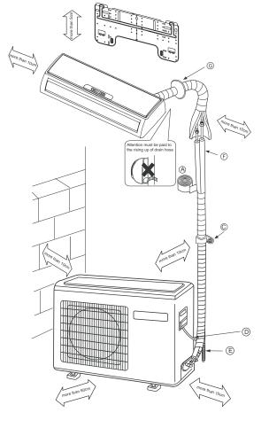
Note: Cooling only units don't have Drain-elbow
