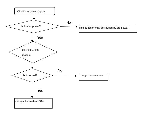
About how to check the IPM module, please refer to IPM protection fault
