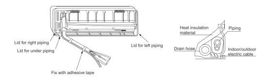
• Indoor/outdoor electric cable and drain hose must be bound with refrigerant piping by protecting tape.
