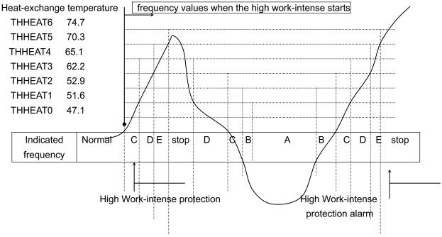
High Work-intense protection alarm will start if there are two times of high work-intense protection within 30 minutes.
