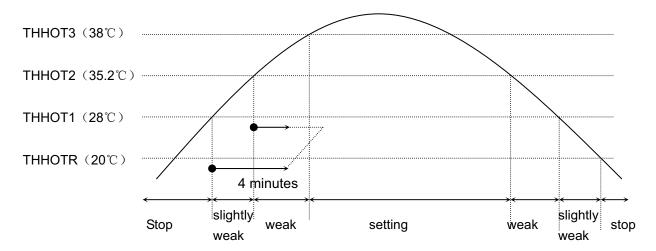
To control the indoor fan motor as shown in the table above according to the heat exchange temperature
