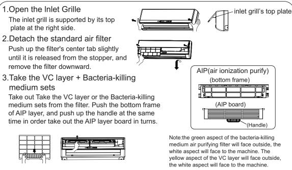
The installation of AIP layer, VC layer + Bacteria-killing medium sets (must be installed)
