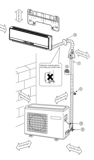
% The marks from (Ato) in the figure are the parts numbers.% The distance between the indoor unit and the floor should be more than 2m.
