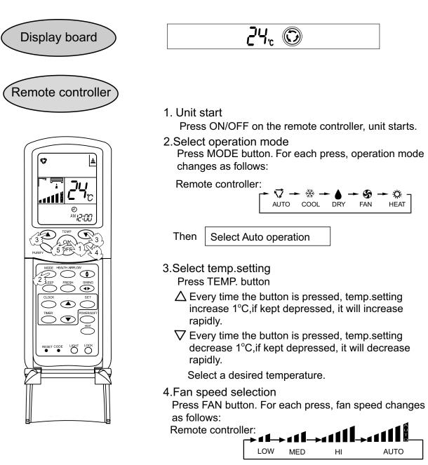
Air conditioner is running under displayed fan speed. When FAN is set to AUTO, the air conditioner automatically adjusts the fan speed according to room temperature.
