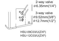
When connecting pipe exceeds 5 meters, 16g refrigerant shall be added per exceeding meter. Charge according to the following list.
