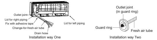
See the Installation from the fresh air sets for the installation of outdoor unit.
