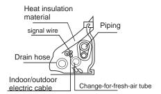
• Indoor/outdoor electric cable and drain hose must be bound with refrigerant piping by protecting tape.
