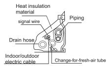
• Indoor/outdoor electric cable and drain hose must be bound with refrigerant piping by protecting tape.
