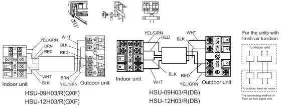
Connecting wiring:  $\geq$  5G1.0mm<sup>2</sup>+1x0.75mm<sup>2</sup>
