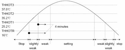
To control the indoor blower fan as shown in the table above according to the heat exchange temperature
