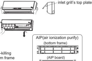
Note:the green aspect of the bacteria-killing medium air purifying filter will face outside, the white aspect will face to the machine. The yellow aspect of the VC layer will face outside, the white aspect will face to the machine.
