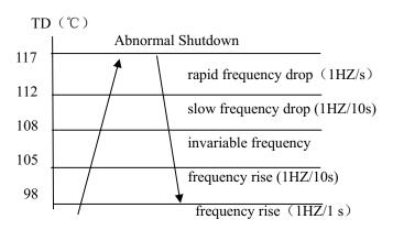
When TD>117°C for 20s continuously, air discharge overheat protection will be activated and fault will be reported to indoor unit.
