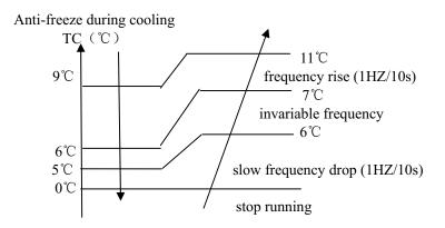
When  $T_C \ \langle \ 5^{\circ}C \$ , compressor frequency will drop at a speed of 1HZ/10s
