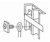
Wiring Method for Ring Terminal Block
