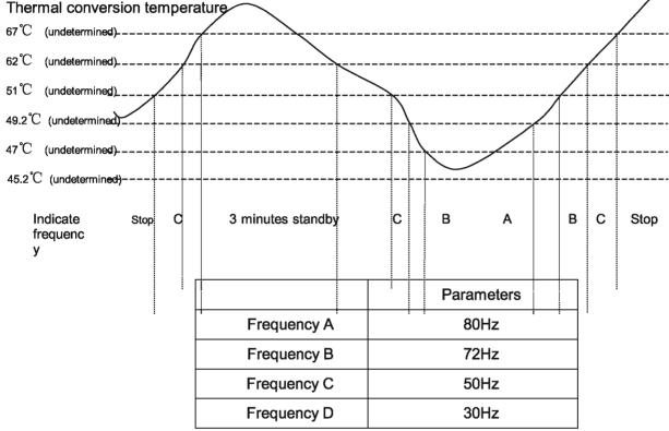
When high-load protection is limited to act twice within 30 minutes, it is high-load protection alarm. When indoor coil pipe temperature is lower than 45°C, it comes back to normal control. The frequency of high load protection is priority.
