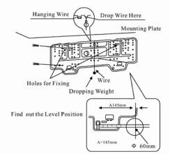
1.Fix the Mounting Plate and Localize the Wall-through Hole
