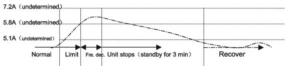
Is this case occurs twice in 30 min, alarm will generate for AC over-current protection.
