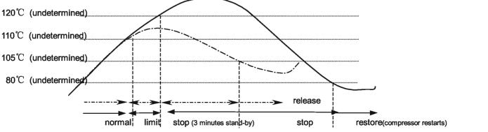
If the compressor continuously stops twice within 30 minutes, the compressor discharge temperature protection alarms.
