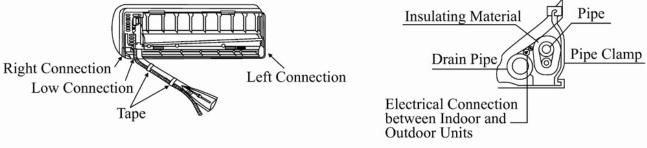
Installation of the Connection Pipe Clips(Left or Left-Back Connection):
