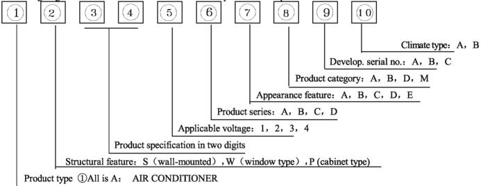
E.g.: in AS102AHAIA, "A" represents air conditioner; "S" means wall mounted indoor unit; "10" indicates cooling capacity of 10000BTU/h; "2" means applicable voltage of 220-230V/50Hz; "A" represents single split system; "H" is for appearance characteristics; "A" means heat pump type and refrigerant of R22; "I" is development serial number; "A" represents climate type.
