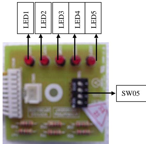
SW05 is used for factory quality control engineers, the default position is : OFF OFF OFF OFF
