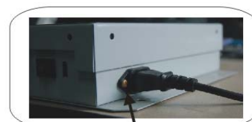
Power Supply(AC220V/50Hz) Powe line (Prefabrication)
