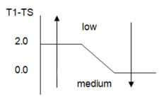
When T1-Ts>2°C, the indoor fan will run at low speed.
