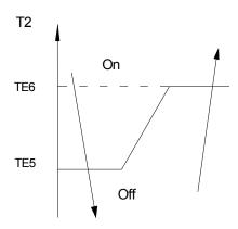
When the evaporator coil temp.T2 keeps lower than TE5 for 5 minutes, the compressor and outdoor fan will shut off. When T2 is higher than TE6, the compressor and outdoor fan will restart up.
