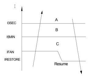
A zone: The current exceeds I<sub>3SEC</sub> for 5 seconds, the compressor and outdoor fan will shut off.
