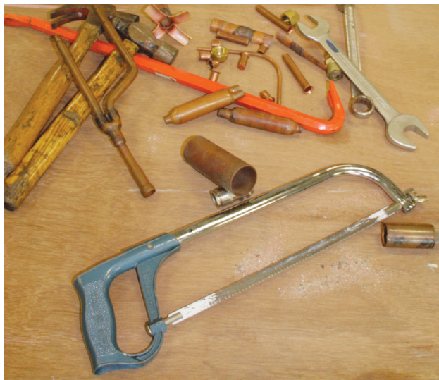
An actual example of cutting copper tubes with a hack saw instead of a regular tube cutter.
