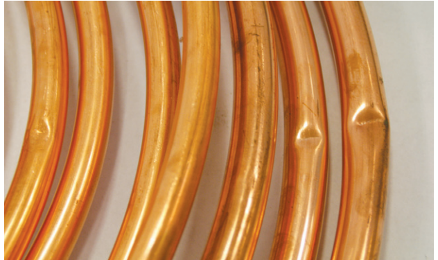
Even little stress can damage and deform the tube walls due to weakness.
