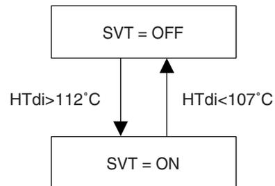
HTdi: Correction value of the discharge pipe temperature on the INV compressor.
