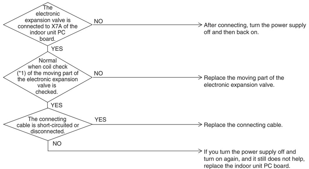
**Note** \*1: Coil check method for the moving part of the electronic expansion valve
