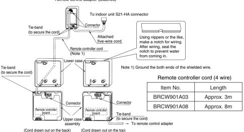
4. Placing the upper case assembly of the remote controller and the upper case of the remote controller adapter back in position
