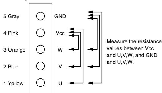
**Check No. 2****Check on pulse input of position signal of fan inverter PC board**
