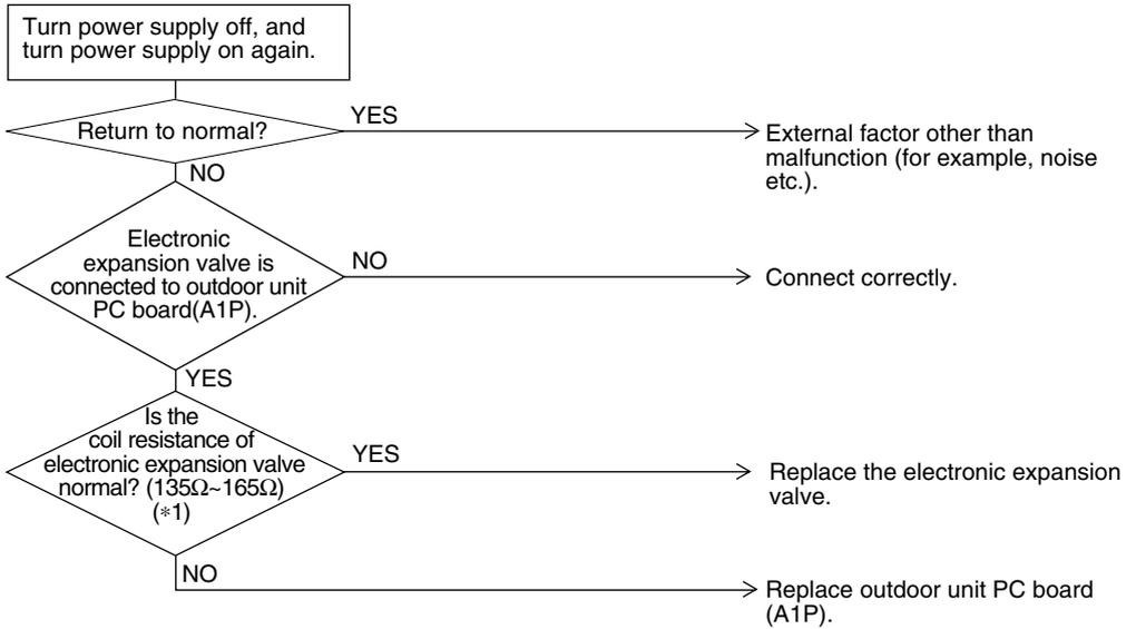
\*Make measurement of resistance between the connector pins, and then make sure the resistance falls in the range of 135 ~ 165Ω.
