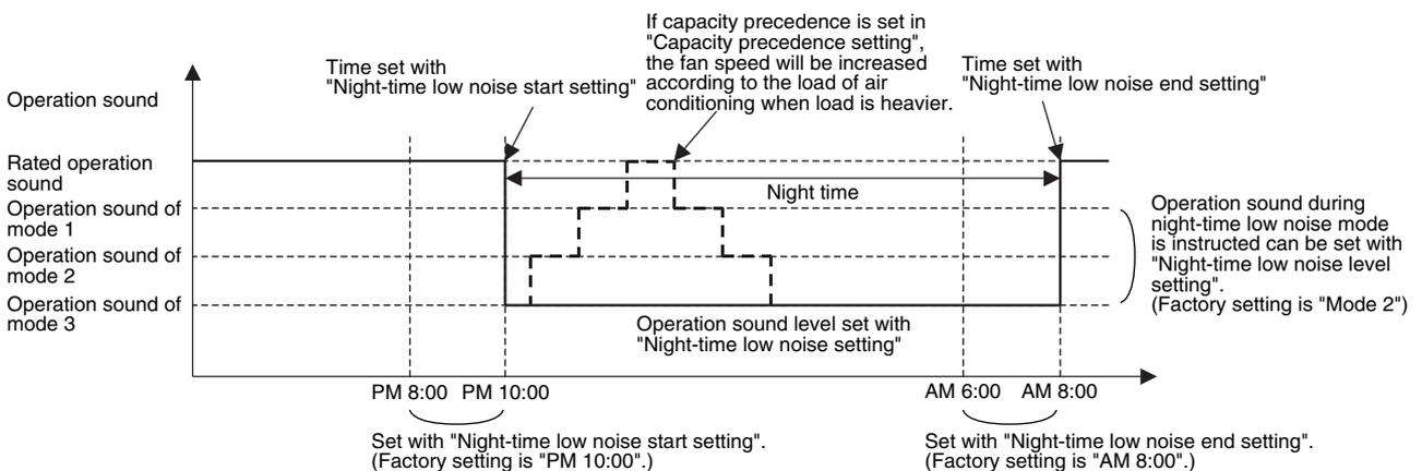
\* "Start time" and "End time" must be regarded as a guide because they are estimated based on the outside air temperature.
