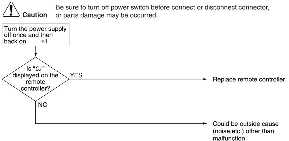
\*1. To delete this, press "Start/ Stop" button for 5 seconds in the check mode of the remote controller.
