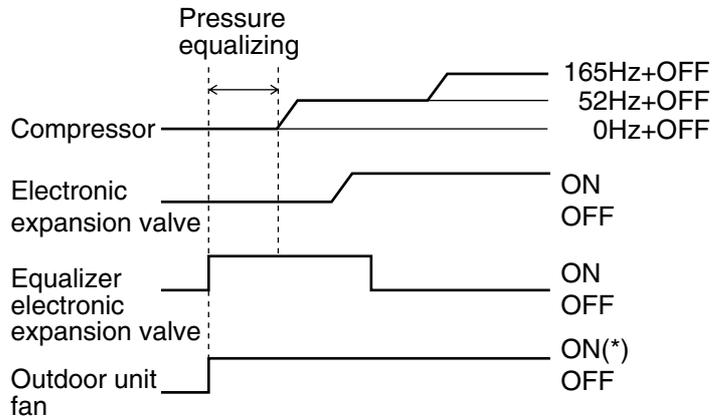
\* According to startup condition, the outdoor unit fan may be turned OFF.
