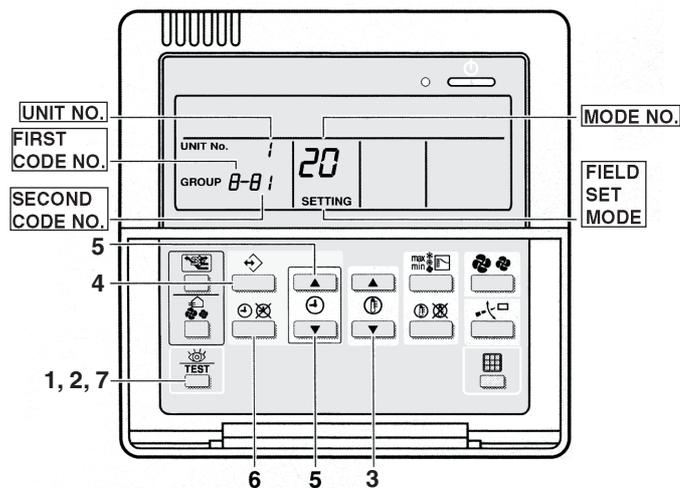
1. When in the normal mode, press the “
