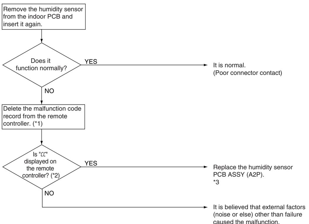
\*1: To delete the record, the **ON/OFF** button of the remote controller must be pushed and held for 5 seconds in the check mode.
