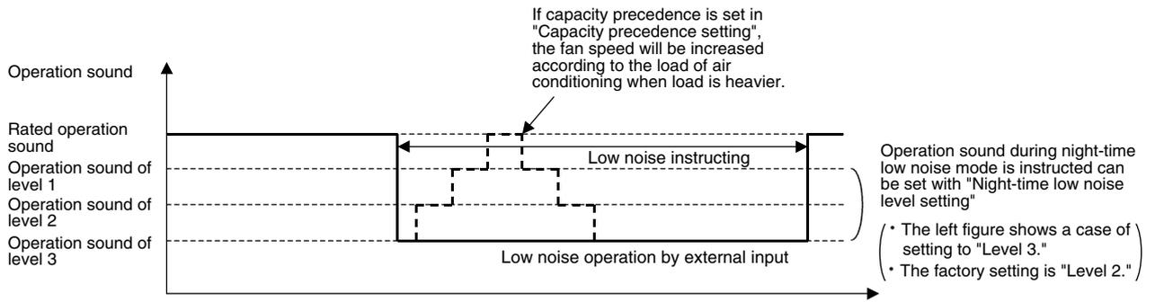
■ Image of "Low noise operation" by external input + operation during "Nighttime low noise setting" and "Required capacity prior" set by remote controller
