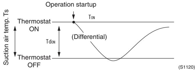
1. Thermostat ON point ( $T_{ON}$ ) according to suction air temp. ( $T_s$ ).
