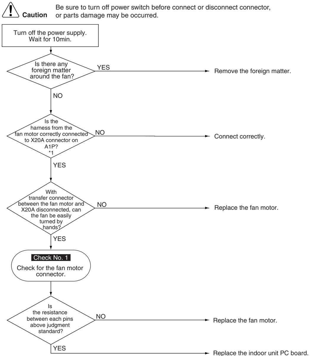
\*1 When there is a relay connector between the connector (X20A) on the indoor PC board and the fan motor, check if the relay connector is correctly connected.
