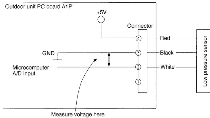
\*2: "Pressure Sensor", pressure/voltage characteristics table.
