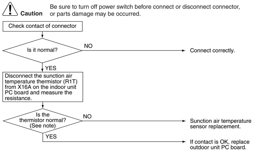
★See **Check No. 6** for “Thermistor temperature/Resistance characteristics”.
