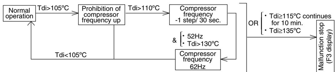
Tdi: Inverter compressor discharge pipe temperature (°C)
