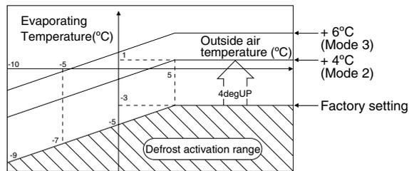
When defrosting conditions are met during heating operation, the indoor unit is demanded defrosting and the following control is performed:
