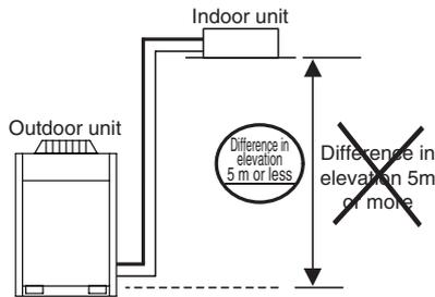
When the indoor unit is installed in a lower position
