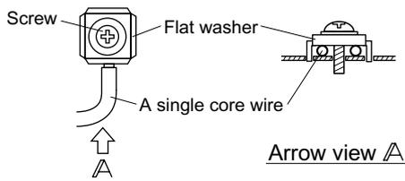
2) Use the following method when installing the round crimp-style terminal.
