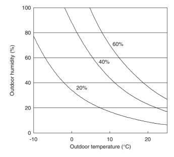
Condition; Model:FTXR28EV1B Indoor temperature setting:20°C Airflow rate:Max Room volume:70m³ Air change rate:0.5/hour humidifying hose length:7.5m
