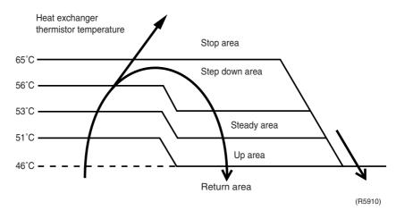
Fig.: Peak-cut control function graph
