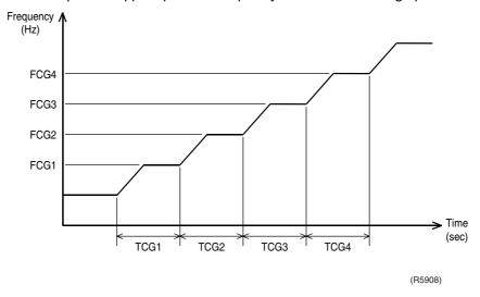
Fig. : Compressor protection function graph.
