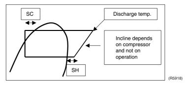
Fig.: Target discharge pipe temperature control graph
