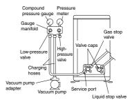
1) Connect projection side of charging hose (which comes from gauge manifold) to gas stop valve's service port.
