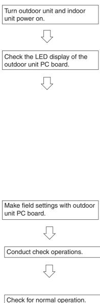
O Be sure to turn the power on 6 hours before starting operation to protect compressors. (to power on clankcase heater)
