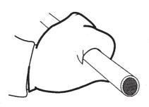
③ Remove the burrs using a file.(Be careful not to let particles enter the pipe.Point the pipe end downward during file
