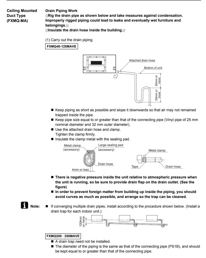
(2) After piping work is finished, check drainage flows smoothly.
