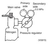
5. Check that the nitrogen is passing through the unit A liquid pipe.
