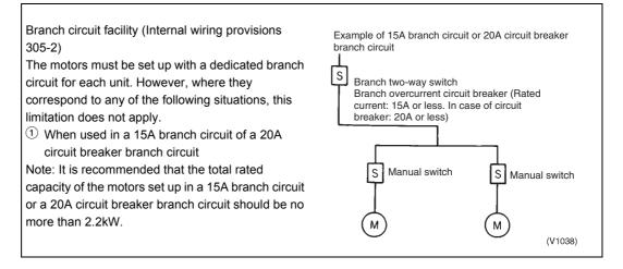
When using high static pressure indoor units the fan motors must have a large capacity. Single phase 220~240V branch circuits are therefore required for each indoor unit.
