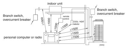
If the electric wave of AM broadcasting is particularly weak, keep distances of 3m or more and use conduit tubes for power and transmission lines.
