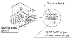
Remove the electric parts box lid, connect a power supply and remote control to the terminals.
