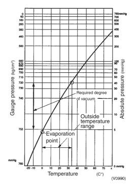
The evacuation of air conditioner piping provides the following effects.
