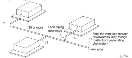
2. The pipework should be kept as short as possible and the number of indoor units per group kept to a minimum.
