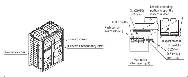
Caution When the 400 volt power supply is applyed to "N" phase by mistake, replace Inverter P.C.B (A2P) and control transformer (T1R, T2R) in switch box together.
