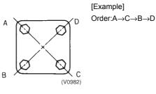
The bolts should be tightened little by little in the above order such that the same degree of torque is applied evenly to each corner.
