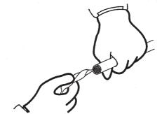
6 Before flaring, clean the cone section of the flaring tool.
