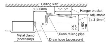
■ If converging multiple drain pipes, install according to the procedure shown below.
