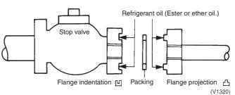
c) Tighten the bolts in opposite corners first to ensure that the connection is true.
