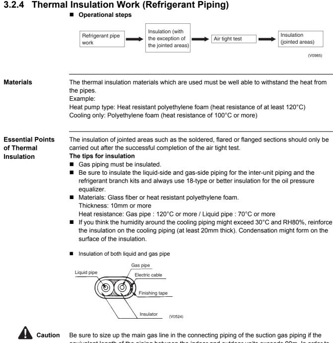
tion Be sure to size up the main gas line in the connecting piping of the suction gas piping if the equivalent length of the piping between the indoor and outdoor units exceeds 90m. In order to minimize the reduction of capacity caused by the pressure drop, the refrigerant pipe size may be sized up.
