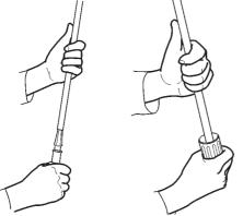
⑤ Clean the inside of the pipe.(Use a thin stick with a cloth wrapped around it.)
