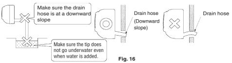
When extending the drain hose, use a commercially available drain extansion hose, and be sure to insulate the extended section of the drain hose which is indoors. (Refer to Fig. 17)
