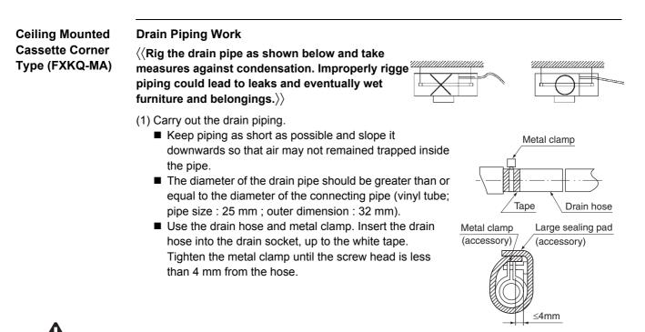
Caution Setting the unit at an angle opposite to the drain piping might cause leaks.
