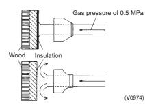
(The nature and amount of the extraneous material inside the pipe can be checked during flushing by placing a rag lightly over the end of the pipe. In the unlikely case that even a small quantity of moisture is found then the inside of the pipe should be dried out thoroughly.) Action:
