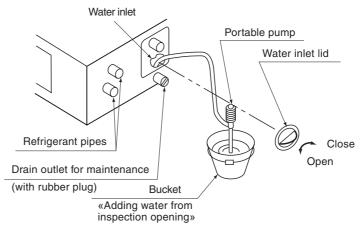
Note: Use this outlet to drain water from the drain pan.
